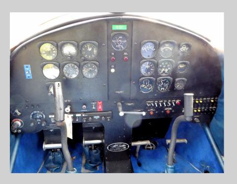
This airplane is unique with "stick" controls instead of the normal control yokes seen on other Spartan Executives. This was a conversion performed in 1952 using the "Field Approval" process.
